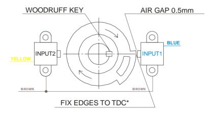
INPUT 1 must be fixed over front upper cylinder as on sketch bellow:
